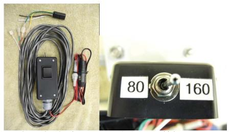
Connect the fused power plug to the 12 volt accessory outlet in your vehicle.
